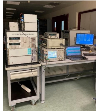
Figure 1. The calibration of KOM 120.1 using the DSWM
